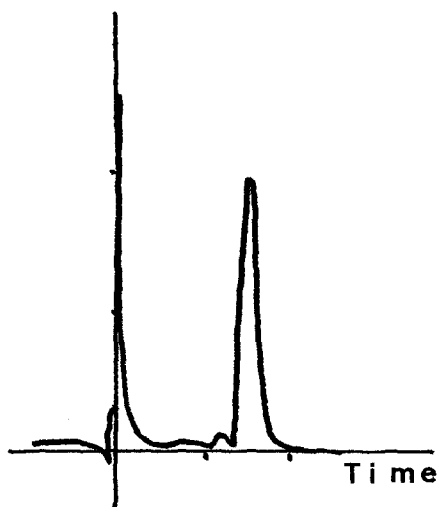
Fig. 1 - Head space gas chromatography of acetaldehyde derived from 45 \mu g of metaldehyde. Column: Porapak T.
